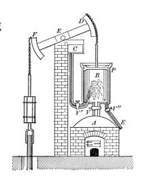
Steam engines were not used to pull trains in those days. The steam engines they had were not strong enough for that. But they were used all over the country for pumping water out of mines. Mines were often flooded with water. The steam engines pumped out the water so the miners could carry on working.
