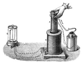
the battery, current was induced in the other direction. Faraday therefore concluded that current was induced in the second coil only when the magnetic field through it was changing.
