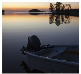
Have you ever been in a small boat? Small boats can be rowed with oars. Sometimes a small boat can have sails. Nowadays a small boat can have an outboard motor. You can see one in the picture. The boat in the picture is not moving. The motor is tilted out of the water. To make the boat go the motor is tilted into the water. Then the motor can turn its propeller. This pushes the boat along.
